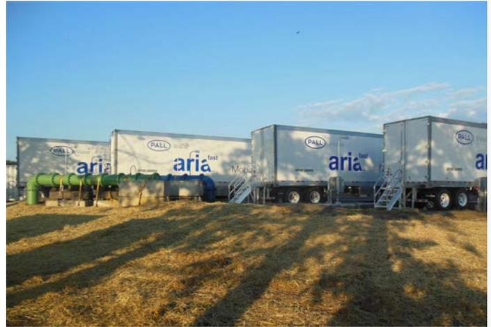
Beyond providing additional capacity to meet peak demand, the fully integrated mobile membrane system's automated process for monthly turbidity monitoring and daily membrane integrity testing have been beneficial for New Jersey American Water. Both processes, which are necessary for compliance, are completed with the touch of a button and results are automatically compiled into a data log.
